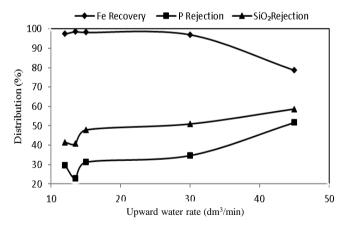
Fig. 8. Effect of water flow rate on iron recovery in underflow and distribution of silica and phosphorus in overflow
