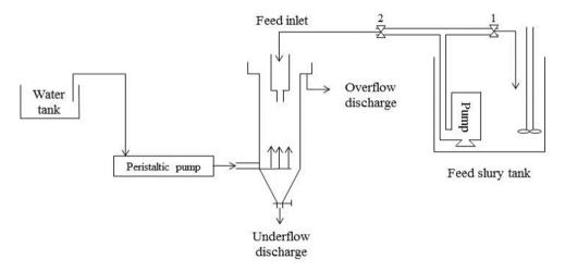
Fig. 5. A schematic diagram of hydroseparator test rig
